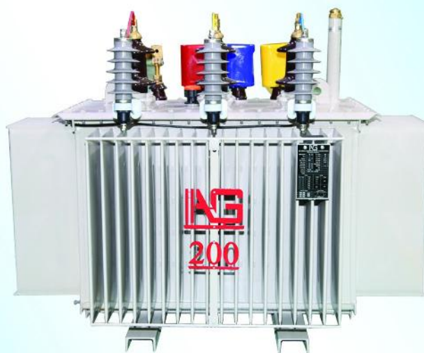
200 kVA, 11/0.4 kV, NLTC -7 Pole Mounted Transformer
